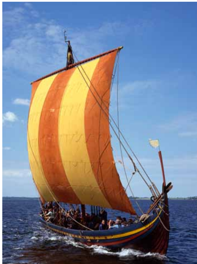
The Sea Stallion, a reconstruction of the warship Skuldelev 2. This great warship was rigged with over 2 km of cordage. She carried an enormous sail, estimated to be 112 m 2 and woven with some 200 kg of wool or flax.
