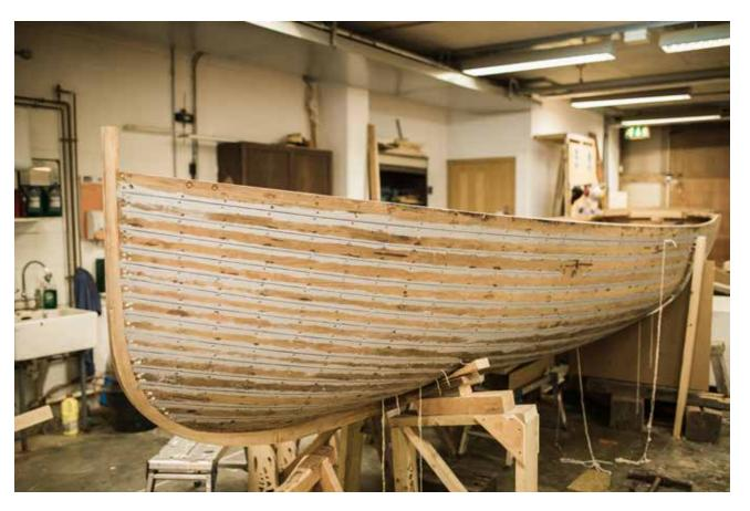
mma is a 22ft x 6ft teak-built steam launch. Although the original builder is unknown, she's believed to have been built around around 1912. Emma is strongly constructed and has a wider beam than one would normally associate with a river or lake vessel. This is fortunate because it will make her well suited for use on the relatively sheltered waters of the Fal estuary.
